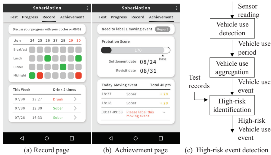
Fig. 3. App pages showing (a) recent test results; (b) overall testing achievements; and (c) sequence of steps used to detect high-risk vehicle use events.
